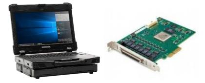
Dualos Link 16 1553 Systems are high-performance portable I/O systems designed for lab and rugged environments. These systems can be a tablet, notebook, laptop or all-in-one unit with ARINC 429, ARINC 664, Mil-Std-1553 or various other I/O and software integrated into the system. They can be standalone analyzers or set-up as general I/O systems.
