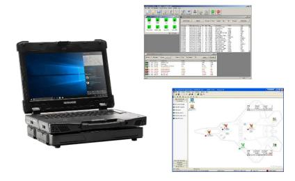
Dualos Standalone Systems are high-performance portable I/O systems designed for lab and rugged environments. These systems can be a tablet, notebook, laptop or all-in-one unit with ARINC 429, ARINC 664, Mil-Std-1553 or various other I/O and software integrated into the system. They can be standalone analyzers or set-up as general I/O systems.
