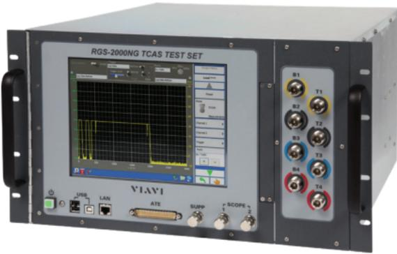
The RGS-2000NG TCAS Test Set is an RF signal generator/receiver for testing Traffic Alert and Collision Avoidance Systems (TCAS) with an option available for testing transponder LRUs. The RGS-2000NG was designed with modern software-driven digital modulation technology and is the RGS-2000 replacement for engineering development, design validation, manufacturing and return-to-service testing.
