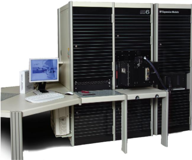
A library of TPS solutions has been developed by VIAVI that will test the full range of navigation, communication, TCAS, transponder, and other RF systems. The product strategy has full OEM support and CMM listing.
