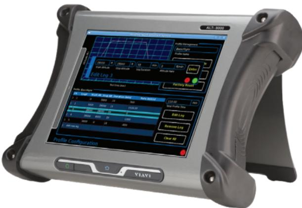
The VIAVI ALT-8000 is the world's first RF-based portable radio altimeter flight line test set. The ALT-8000 tests from the TX/RX antennas to the indicator in the cockpit, allowing the operator to replicate in-flight conditions and isolate a bad component of the installed system.
