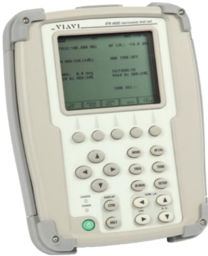
The VIAVI IFR4000 Flight Line Test Set is designed for testing ILS, VOR, Marker Beacon, HF/VHF/UHF Communications (NAV/COMM) Systems, and ELT Short Range Emergency Beacons and 406 MHz COSPAS/SARSAT Long Range Emergency Beacons. The menu-driven functionality and guided test capability make this instrument extremely easy to use.
